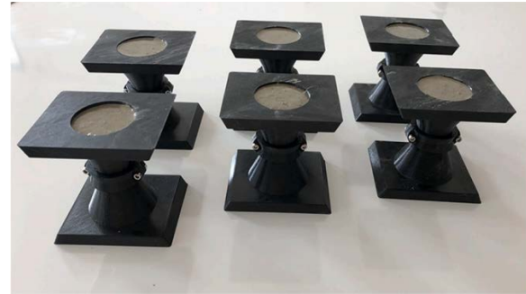
Figure 2.7: Double Dumbbell device filled with mortar and in the testing equipment. Taken from [17].
