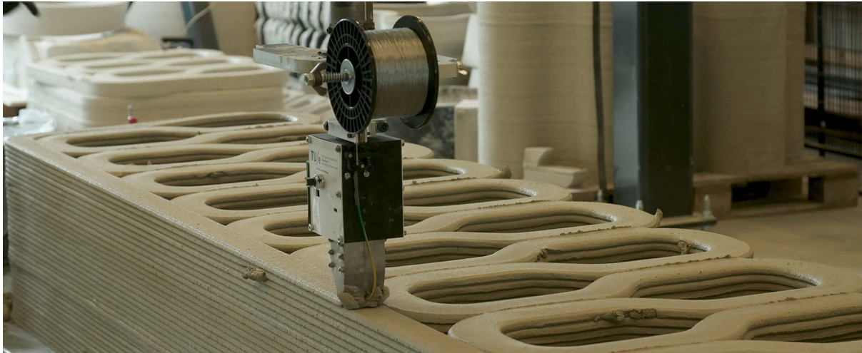
Figure 4.11: Reinforcement Entrainment Device (RED) developed at TU Eindhoven to add steel cable reinforcement into the printed concrete
