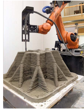
Figure 3.3: Left: ABB robotic arm mounted on a fixed base at Tallinn University of Applied Sciences used for educational and research-scale 3D concrete printing [52]. Right: KUKA robotic arm system at Hyperion Robotics in Finland used for automated fabrication of reinforced concrete elements [53].
