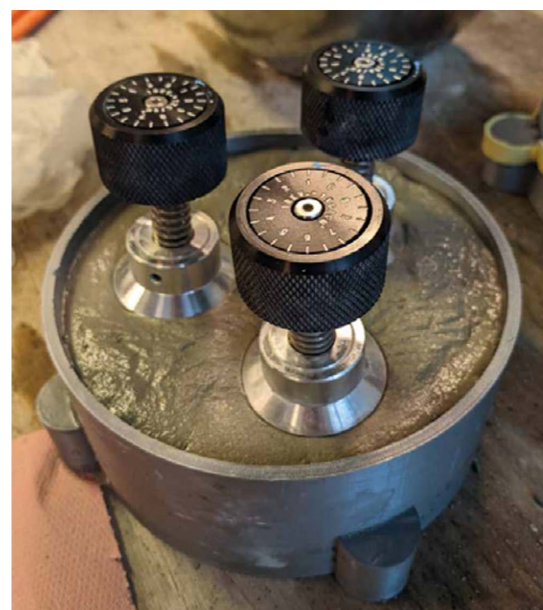
Figure 2.9: A pocket shear vane HumboldtH-4212MH, images taken from [26].
