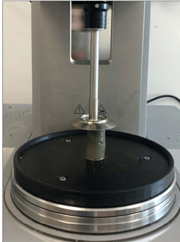
Figure 2.4: Squeeze flow test, taken from [17].
