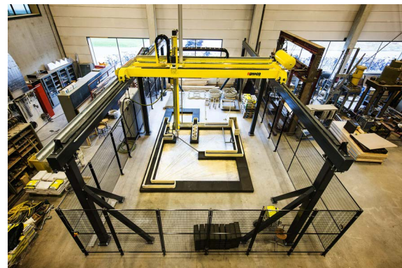
Figure 3.2: Examples of Cartesian gantry-type 3D concrete printers. Left: a COBOD system configured for full-scale on-site printing [51]. Right: large-scale gantry at TU/e 3DCP research laboratory
