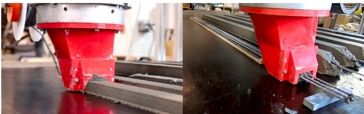
Figure 4.12: Integration of mineral-impregnated carbon-fibre (MCF) rovings into the extrusion process, taken from [97]
