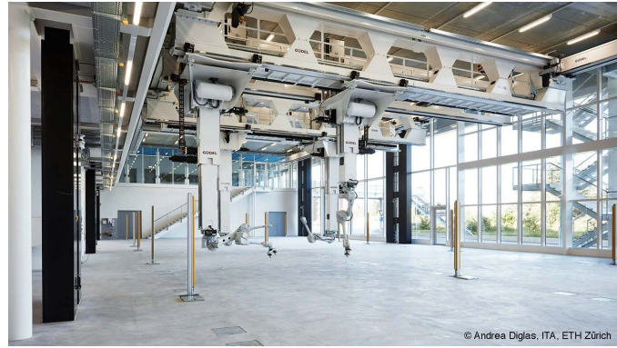
Figure 3.5: Left: COBOD BOD2 system at TU Braunschweig equipped with a vertical telescopic unit and rotating robotic arm enabling multifunctional printing and shotcrete (SC3DP) operations [56]. Right: ETH Zurich's Robotic Fabrication Laboratory (RFL) with an overhead gantry and four six-axis robots operating within a 43 \times 16 \times 8 m workspace [57].
