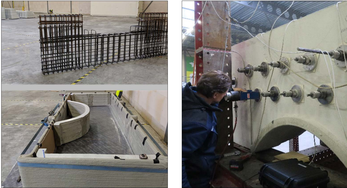
Figure 3.22: Reinforced anchor blocks were cast in 3D-printed formwork, and post-tensioning of tendons.
