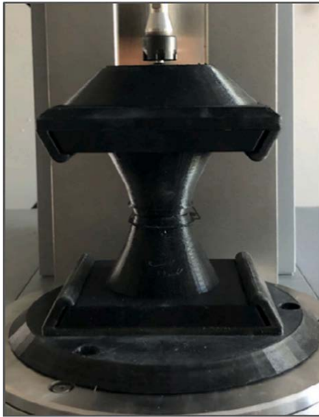
Figure 2.7: Double Dumbbell device filled with mortar and in the testing equipment. Taken from [17].
