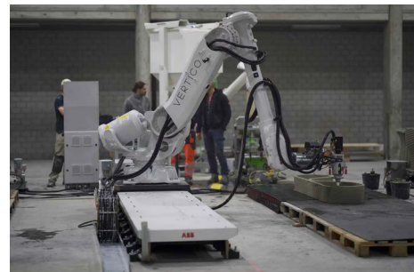
Figure 3.4: Left: Robotic arm on linear track at Weber Beamix Print fabriek used for industrial-scale 3D concrete printing [54]. Right: Vertico print facility at TU/e featuring a KUKA robotic arm on a movable track for printing curved and overhanging geometries [55].
