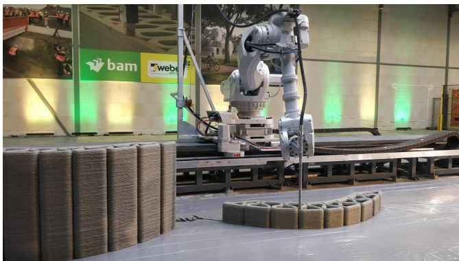
Figure 3.4: Left: Robotic arm on linear track at Weber Beamix Print fabriek used for industrial-scale 3D concrete printing [54]. Right: Vertico print facility at TU/e featuring a KUKA robotic arm on a movable track for printing curved and overhanging geometries [55].
