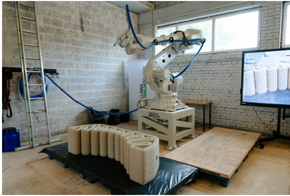
Figure 3.3: Left: ABB robotic arm mounted on a fixed base at Tallinn University of Applied Sciences used for educational and research-scale 3D concrete printing [52]. Right: KUKA robotic arm system at Hyperion Robotics in Finland used for automated fabrication of reinforced concrete elements [53].
