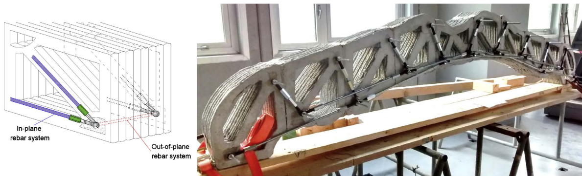
Figure 4.6: External reinforcement strategies for 3D-printed concrete. Left: in-plane and out-of-plane rebar systems that can be attached externally to enhance structural capacity. Right: an optimised 3D-printed beam with a variable cross-section demonstrating how geometry can be tailored to structural demand, taken from [88].
