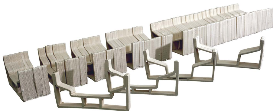
Figure 5.31: 3d printed clay formwork. Taken from [60].
