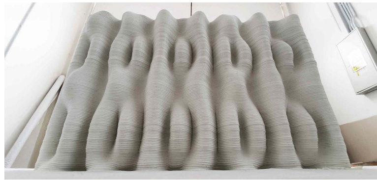
Figure 3.2: Comparison of traditional crinkle-crankle wall (left) and a digitally fabricated wavy 3DCP wall (right). Crinkle-crankle wall: a traditional wavy brick wall design that achieves stability through its serpentine form while using fewer bricks compared to a straight wall. Courtesy to [34]. Wavy 3DCP wall: parametric concrete wall form generated using computational design. Courtesy to [35].
