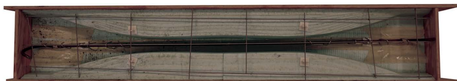
Figure 5.29: CNC milled expanded polystyrene formwork. Taken from [60].
