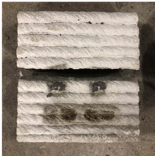
Figure 2.9: Interlayer delamination, after fire testing, taken from [7].
