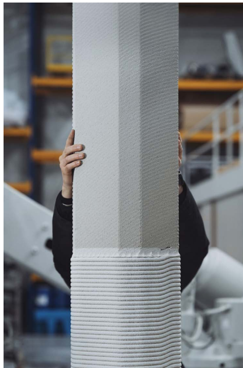
Figure 2.16: Structure of a milled surfaced after printing, by Vertico.
