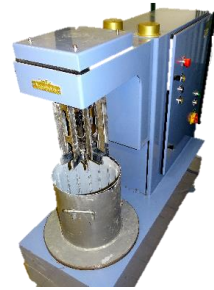
Figure 2. Commonly used vane-in-cup rheometers for 3D concrete printing.
