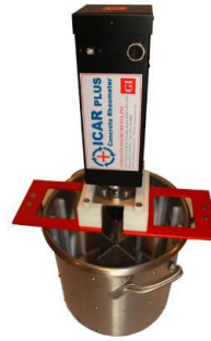
Figure 2. Commonly used vane-in-cup rheometers for 3D concrete printing.
